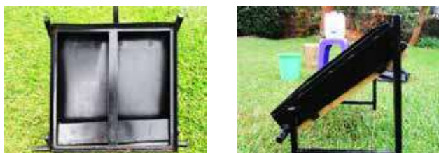
Figure 5. Fabricated solar distiller with inlet pipes, outlet pipes and water collection gutters
