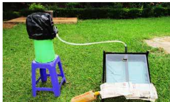
Figure 6. Fully assembled solar distiller with secondary heating and cooling components
