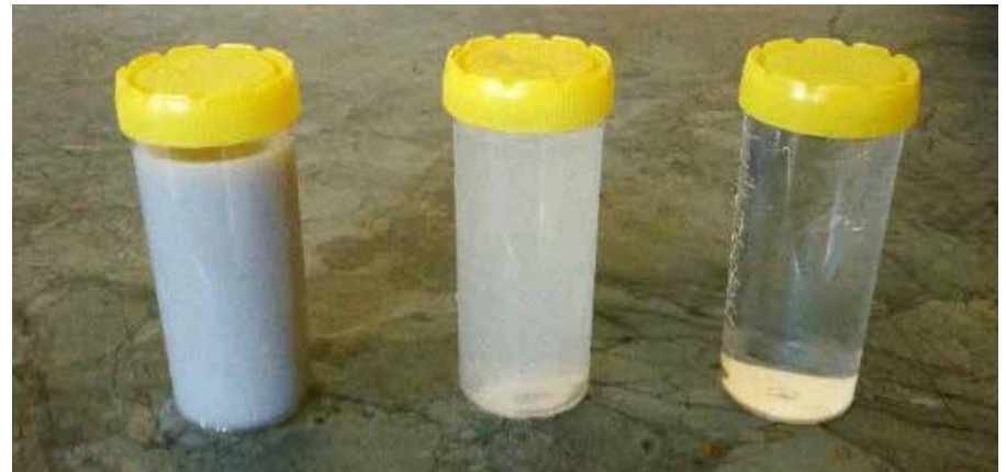
Figure 5: Showing the samples of wastewater from the mixing, sedimentation and filtration units
