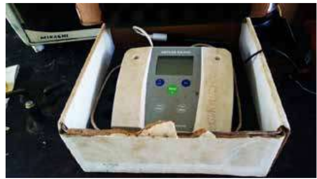
Figure 7. Conductivity meter for taking measurements of totally dissolved solids, conductivity, salinity and temperature
