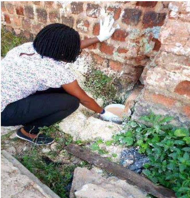
Figure 2: Determining the flow rate using the bucket method.
