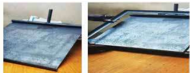
Figure 4. Partially fabricated metal solar distillation basin with feedwater distribution pipe
