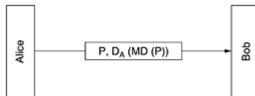
Figure 8-20. Digital signatures using message digests.
