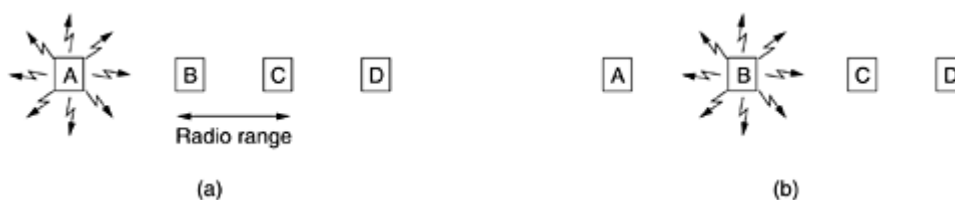
Figure 4-11. A wireless LAN. (a) A transmitting. (b) B transmitting.
