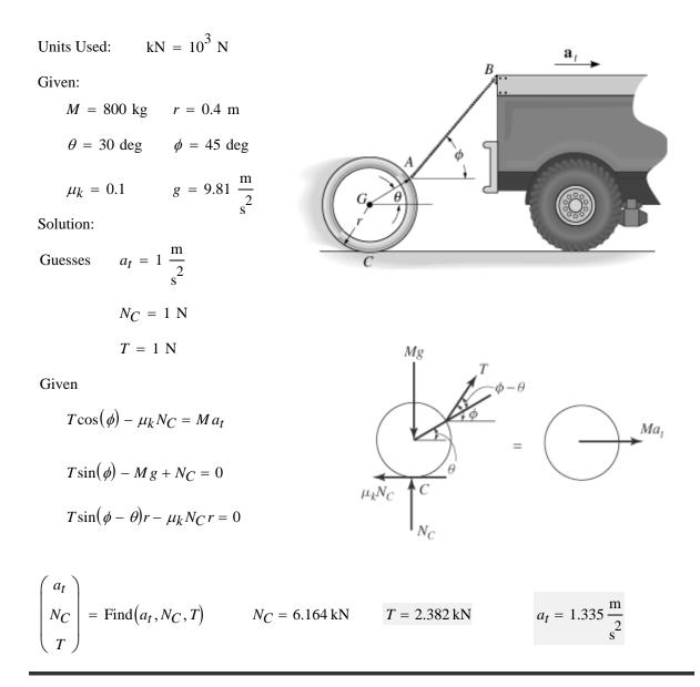
The pipe has a mass M and is held in place on the truck bed using the two boards A and B. Determine the acceleration of the truck so that the pipe begins to lose contact at A and the bed of the truck and starts to pivot about B. Assume board B will not slip on the bed of the truck, and the pipe is smooth. Also, what force does board B exert on the pipe during the acceleration?
