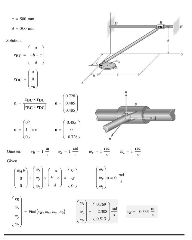
The rod *AB* is attached to collars at its ends by ball-and-socket joints. If collar *A* has a speed  $v_A$ , determine the speed of collar *B* at the instant shown.
