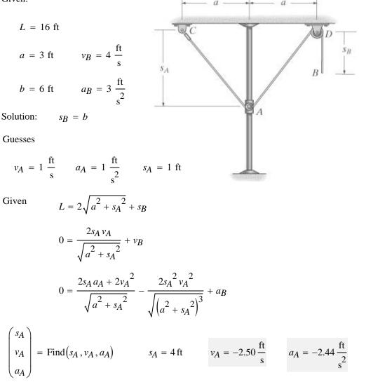
The crate *C* is being lifted by moving the roller at *A* downward with constant speed  $v_A$  along the guide. Determine the velocity and acceleration of the crate at the instant  $s = s_I$ . When the roller is at *B*, the crate rests on the ground. Neglect the size of the pulley in the calculation. *Hint:* Relate the coordinates  $x_C$  and  $x_A$  using the problem geometry, then take the first and second time derivatives.
