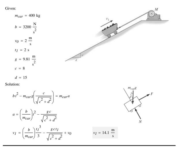
The mine car of mass  $m_{car}$  is hoisted up the incline using the cable and motor M. For a short time, the force in the cable is  $F = bt^2$ . If the car has an initial velocity  $v_0$  when t = 0, determine the distance it moves up the plane when  $t = t_1$ .
