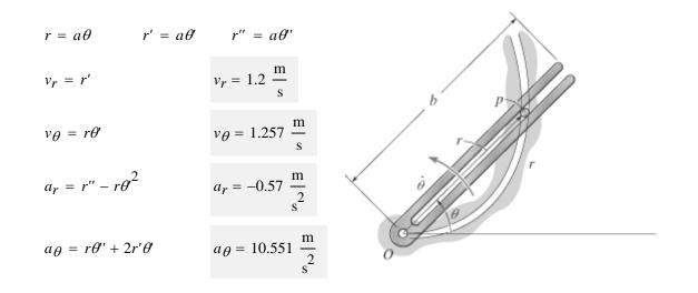
The slotted link is pinned at *O*, and as a result of the constant angular velocity  $\theta$  it drives the peg *P* for a short distance along the spiral guide  $r = a\theta$  where  $\theta$  is in radians. Determine the velocity and acceleration of the particle at the instant it leaves the slot in the link, i.e., when r = b.
