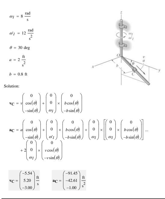
At the instant shown, the arm *OA* of the conveyor belt is rotating about the z axis with a constant angular velocity  $\omega_1$ , while at the same instant the arm is rotating upward at a constant rate  $\omega_2$ . If the conveyor is running at a constant rate r' = v, determine the velocity and acceleration of the package *P* at the instant shown. Neglect the size of the package.
