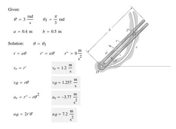
The slotted link is pinned at *O*, and as a result of the angular velocity  $\theta$  and the angular acceleration  $\theta'$  it drives the peg *P* for a short distance along the spiral guide  $r = a\theta$ . Determine the radial and transverse components of the velocity and acceleration of *P* at the instant  $\theta = \theta_I$ .
