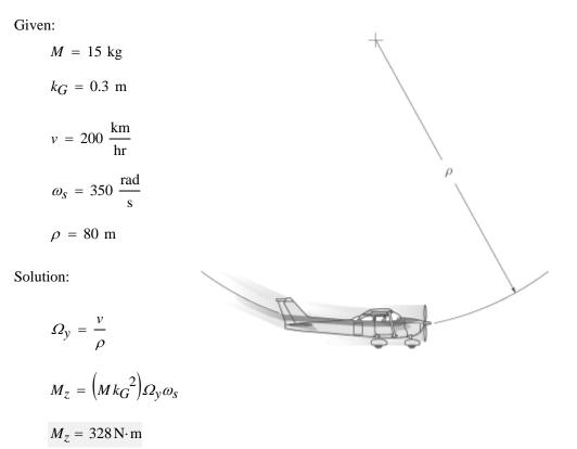
The rotor assembly on the engine of a jet airplane consists of the turbine, drive shaft, and compressor. The total mass is  $m_r$ , the radius of gyration about the shaft axis is  $k_{AB}$ , and the mass center is at *G*. If the rotor has an angular velocity  $\omega_{AB}$ , and the plane is pulling out of a vertical curve while traveling at speed *v*, determine the components of reaction at the bearings *A* and *B* due to the gyroscopic effect.
