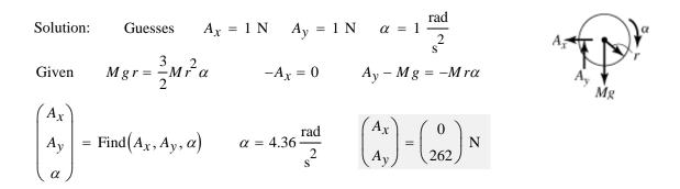
The wheel of mass  $m_w$  has a radius of gyration  $k_A$ . If the wheel is subjected to a moment M = bt, determine its angular velocity at time t starting from rest. Also, compute the reactions which the fixed pin A exerts on the wheel during the motion.
