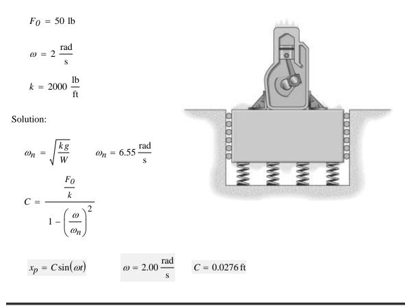
The engine is mounted on a foundation block which is spring-supported. The block and engine have total weight W and the engine, when running, creates an impressed force  $F = F_0 \sin \omega t$ . Assume that the system vibrates only in the vertical direction, with the positive displacement measured downward, and that the total stiffness of the springs can be represented as k. What rotational speed  $\omega$  will cause resonance?
