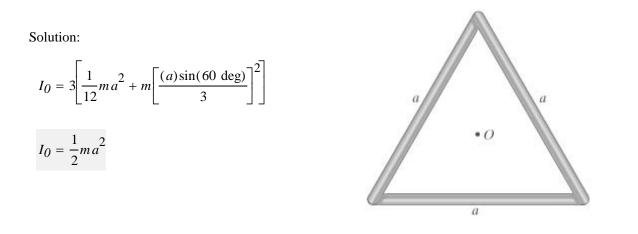
The slender rods have weight density  $\gamma$ . Determine the moment of inertia of the assembly about an axis perpendicular to the page and passing through the pin at A.
