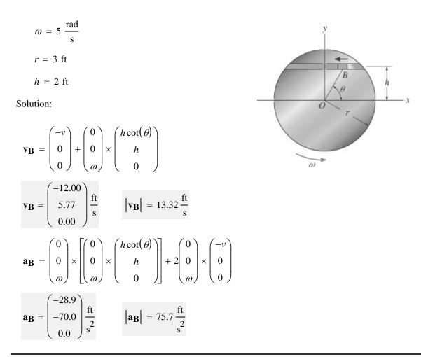
While the swing bridge is closing with constant rotation  $\omega$ , a man runs along the roadway at constant speed *v* relative to the roadway. Determine his velocity and acceleration at the instant shown.
