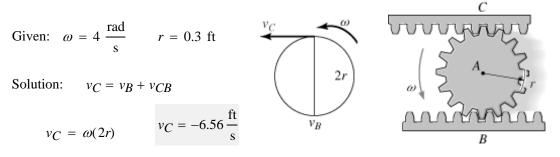
The pinion gear rolls on the gear racks. If *B* is moving to the right at speed  $v_B$  and *C* is moving to the left at speed  $v_C$  determine the angular velocity of the pinion gear and the velocity of its center *A*.
