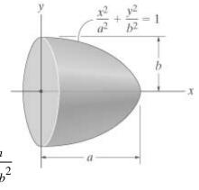
Determine the radius of gyration  $k_x$  of the body. The specific weight of the material is  $\gamma$ .
