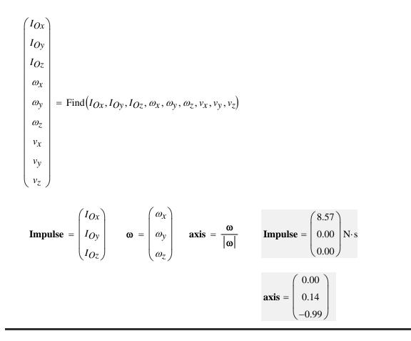
Rod *AB* has weight *W* and is attached to two smooth collars at its ends by ball-and-socket joints. If collar *A* is moving downward with speed  $v_A$  when z = a, determine the speed of *A* at the instant z = 0. The spring has unstretched length *c*. Neglect the mass of the collars. Assume the angular velocity of rod *AB* is perpendicular to its axis.
