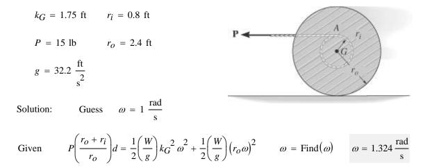
The double pulley consists of two parts that are attached to one another. It has a weight  $W_p$  and a centroidal radius of gyration  $k_0$
