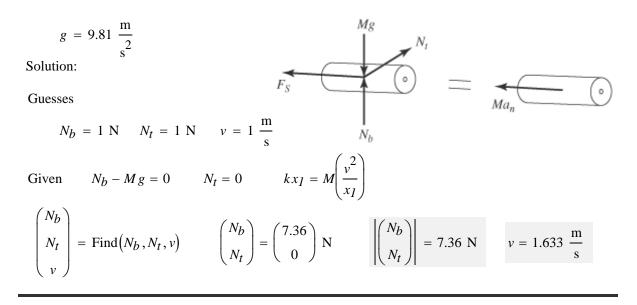
The block has weight W and it is free to move along the smooth slot in the rotating disk. The spring has stiffness k and an unstretched length  $\delta$ . Determine the force of the spring on the block and the tangential component of force which the slot exerts on the side of the block, when the block is at rest with respect to the disk and is traveling with constant speed v.
