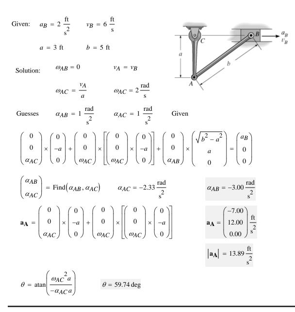
The ends of the bar *AB* are confined to move along the paths shown. At a given instant, *A* has velocity  $v_A$  and acceleration  $a_A$ . Determine the angular velocity and angular acceleration of *AB* at this instant.
