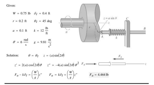
The spring-held follower *AB* has weight *W* and moves back and forth as its end rolls on the contoured surface of the cam, where the radius is *r* and  $z = a \sin(2\theta)$ . If the cam is rotating at a constant rate of  $\theta'$ , determine the maximum and minimum force the follower exerts on the cam if the spring is compressed  $\delta_1$  when  $\theta = 45^\circ$ .
