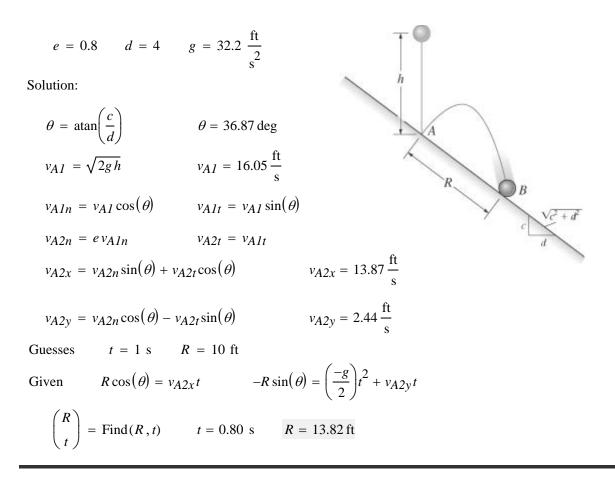
The ball is dropped from rest and falls a distance h before striking the smooth plane at A. If it rebounds and in time t again strikes the plane at B, determine the coefficient of restitution e between the ball and the plane. Also, what is the distance R?
