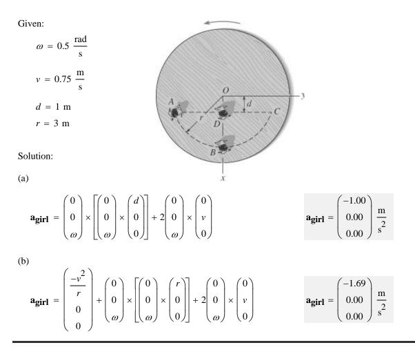
A girl stands at A on a platform which is rotating with angular acceleration  $\alpha$  and at the instant shown has angular velocity  $\omega$ . If she walks at constant speed v measured relative to the platform, determine her acceleration (a) when she reaches point D in going along the path ADC, and (b) when she reaches point B if she follows the path ABC.
