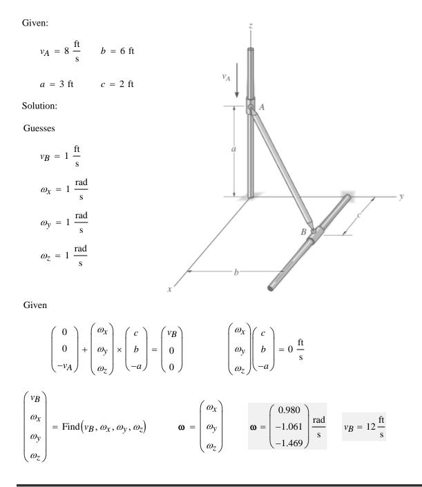
If the collar at A is moving downward with an acceleration  $a_A$ , at the instant its speed is  $v_A$ , determine the acceleration of the collar at B at this instant.
