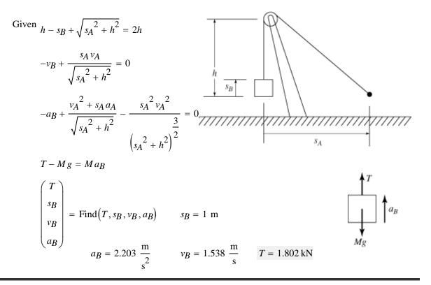
Block *B* has a mass *m* and is hoisted using the cord and pulley system shown. Determine the magnitude of force  $\mathbf{F}$  as a function of the block's vertical position *y* so that when  $\mathbf{F}$  is applied the block rises with a constant acceleration  $a_B$ . Neglect the mass of the cord and pulleys.
