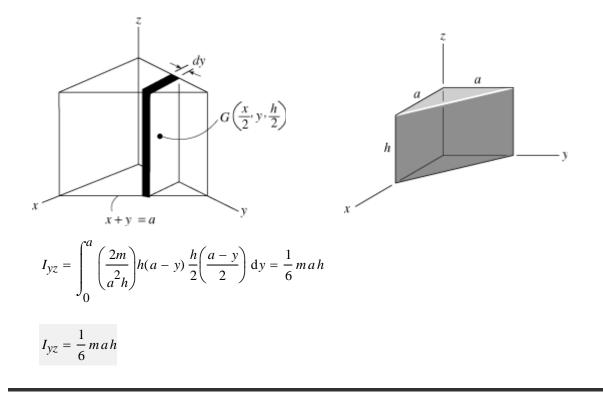
Determine by direct integration the product of inertia  $I_{xy}$  for the homogeneous prism. The density of the material is  $\rho$ . Express the result in terms of the mass *m* of the prism.
