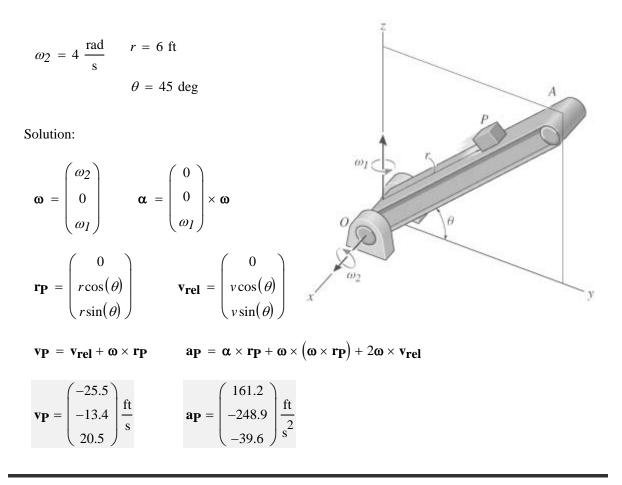
At the instant shown, the arm *OA* of the conveyor belt is rotating about the *z* axis with a constant angular velocity  $\omega_l$ , while at the same instant the arm is rotating upward at a constant rate  $\omega_2$ . If the conveyor is running at the rate r' = v which is increasing at the rate r'' = a, determine the velocity and acceleration of the package *P* at the instant shown. Neglect the size of the package.
