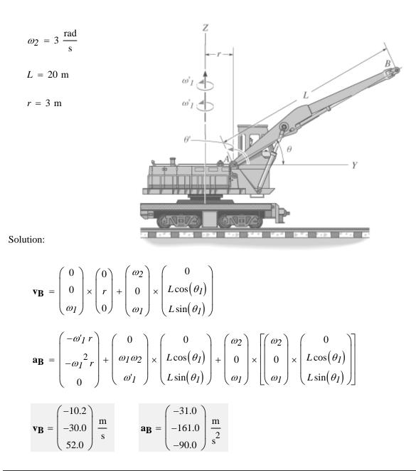
The locomotive crane is traveling to the right with speed v and acceleration a. The boom AB is rotating about the Z axis with angular velocity  $\omega_1$  which is increasing at  $\omega'_1$ . At this same instant,  $\theta = \theta_1$  and the boom is rotating upward at a constant rate of  $\theta' = \omega_2$ . Determine the velocity and acceleration of the tip B of the boom at this instant.
