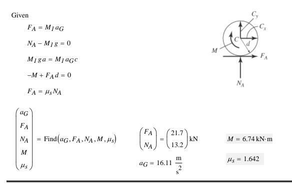
The bicycle and rider have a mass M with center of mass located at G. If the coefficient of kinetic friction at the rear tire is  $\mu_B$ , determine the normal reactions at the tires A and B, and the deceleration of the rider, when the rear wheel locks for braking. What is the normal reaction at the rear wheel when the bicycle is traveling at constant velocity and the brakes are not applied? Neglect the mass of the wheels.
