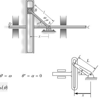
Determine the angular velocity of rod AB for the given  $\theta$ . The shaft and the center of the roller *C* move forward at a constant rate *v*.
