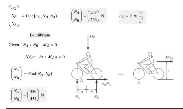
The bicycle and rider have a mass M with center of mass located at G. Determine the minimum coefficient of kinetic friction between the road and the wheels so that the rear wheel B starts to lift off the ground when the rider applies the brakes to the front wheel. Neglect the mass of the wheels.
