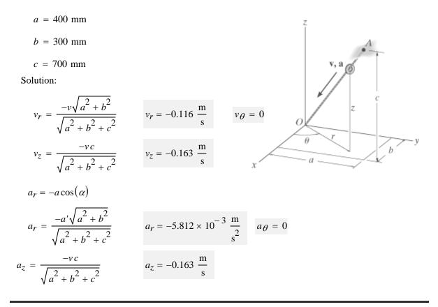
A double collar *C* is pin-connected together such that one collar slides over a fixed rod and the other slides over a rotating rod. If the geometry of the fixed rod for a short distance can be defined by a lemniscate,  $r^2 = (a \cos b\theta)$ , determine the collar's radial and transverse components of velocity and acceleration at the instant  $\theta = 0^\circ$  as shown. Rod *OA* is rotating at a constant rate of  $\theta$ .
