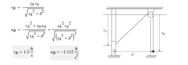
The roller at A is moving upward with a velocity  $v_A$  and has an acceleration  $a_A$  at  $s_A$ . Determine the velocity and acceleration of block B at this instant.
