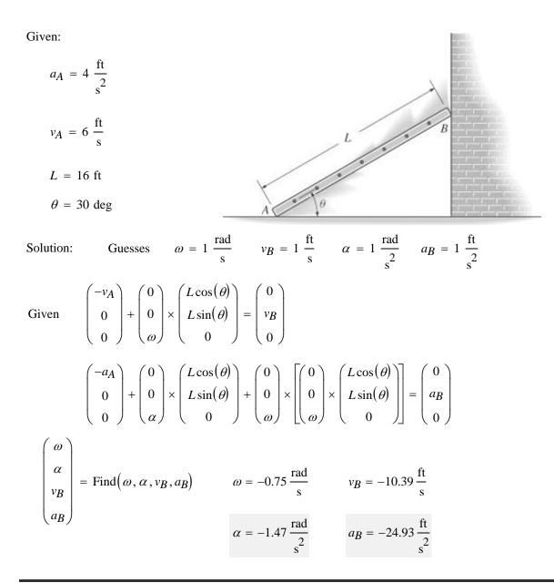
At a given instant the top B of the ladder has acceleration  $a_B$  and
