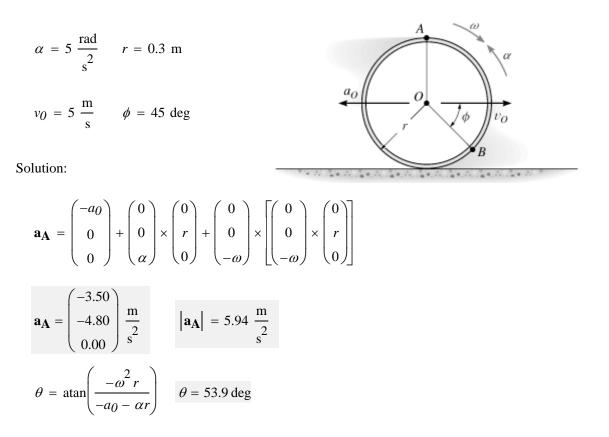
The hoop is cast on the rough surface such that it has angular velocity  $\omega$  and angular acceleration  $\alpha$ . Also, its center has a velocity  $v_0$  and a deceleration  $a_0$ . Determine the acceleration of point *B* at this instant.
